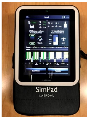
Figure 2. SimPad with SkillReporter. This is connected to the feedback manikin that displays results of the CPR skills assessed.
